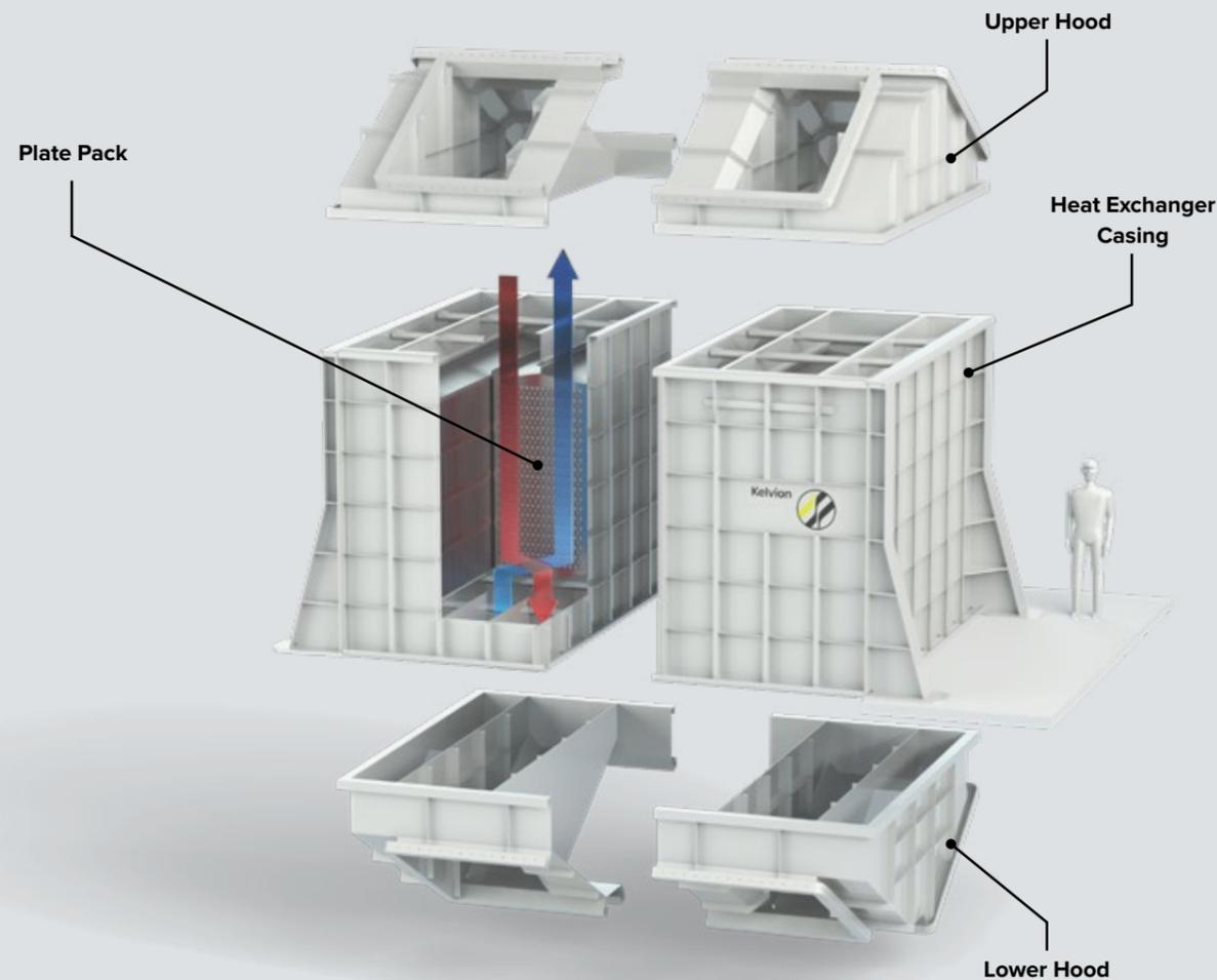
The space-saving design allows fast installation, with short, vertical flow channels to simplify cleaning and can be perfectly adapted to every process-engineering or space situation. Easy handling and considerable potential savings – meaning genuine progress.
