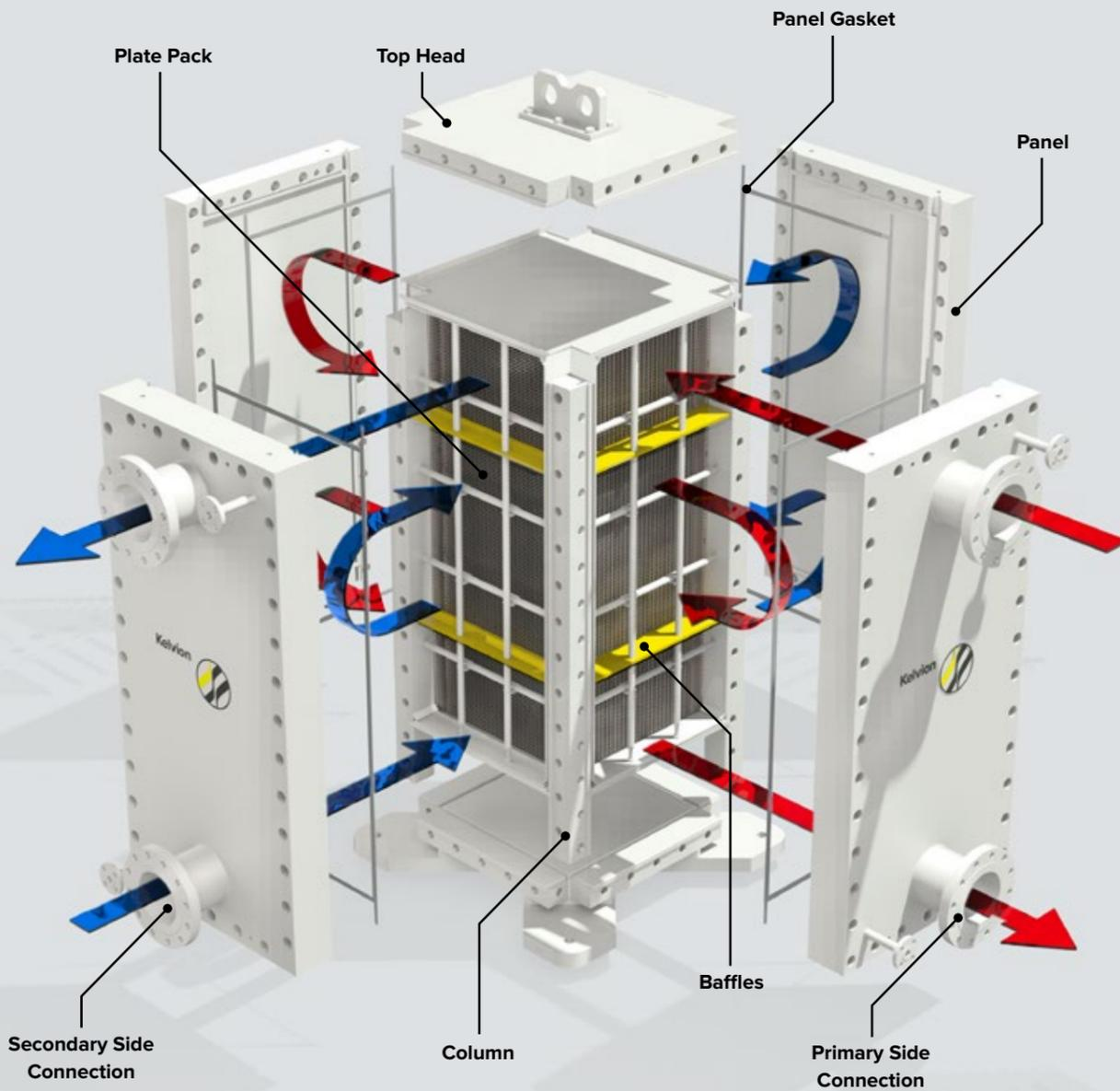
The solidly bolted frame consists of four columns, top and bottom heads as well as four side panels. These side panels can be detached swiftly and allow free access all the way around for the thorough and easy cleaning of the welded plate package.
